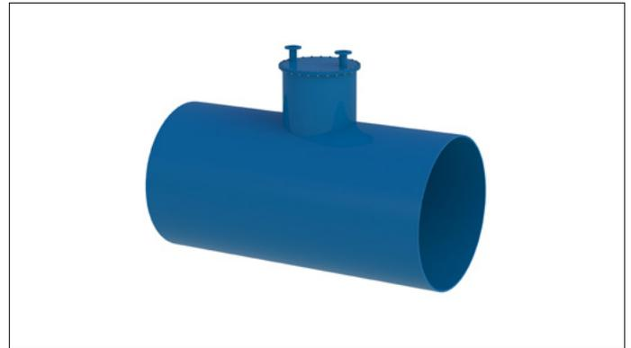
Drag and drop this model onto a pipe of any common diameter and it will automatically create an air-trap, including recommended diameter and height sizing.
