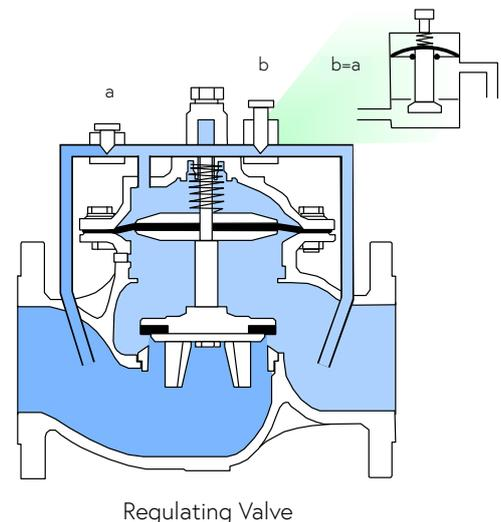
The 2-way control device provides sensitive, accurate, and constant modulating control of the main valve. The main valve does not fully open, as the control device prevents total drainage of the control chamber. The 2-way control device is standard in most pressure regulating valves.
