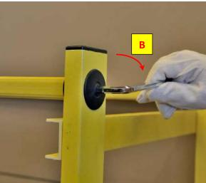
d. Repeat the locking process for the rest 7 rods and plugs.
