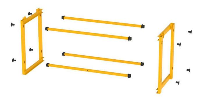
3. Note the skid positioning direction (note the location of the connecting rods sockets) and place the first frame it that direction. Note that the right frame is marked with a green sticker, and the left frame is marked with a red sticker.
