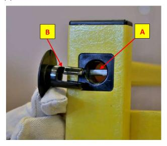
b. Insert the plug to the rod's socket (A) direction, and press it in using the plastic hammer (B).
